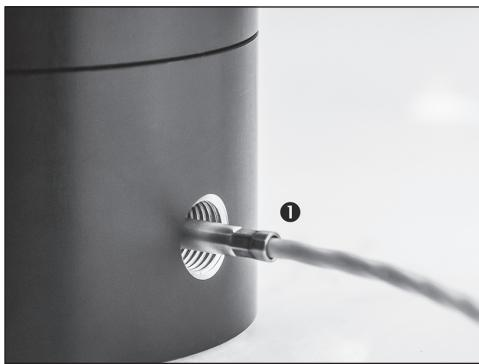
① CalBox with mounted temperature probe
